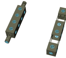
Figure 1: Representation of structural robot. Left : Robot with manipulators fully deployed. Right : Robot with manipulators retracted and main body extended for locomotion.
