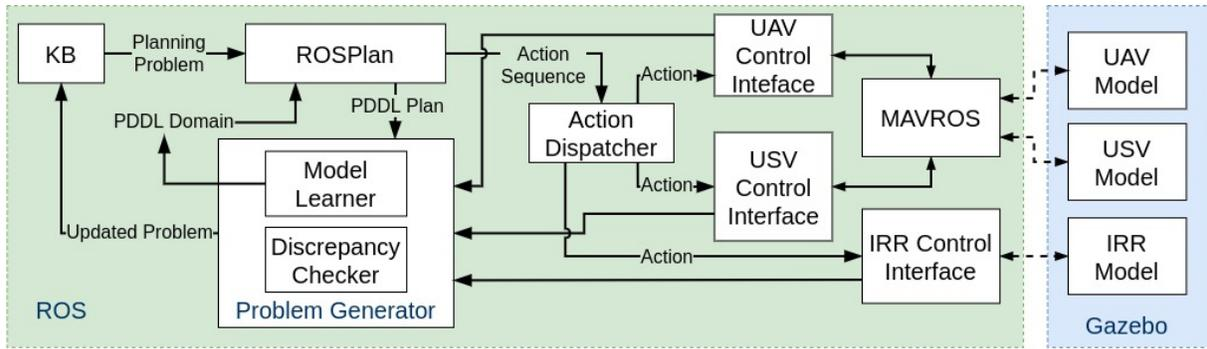
Figure 2: Autonomy architecture for Wind Farm O&M.
